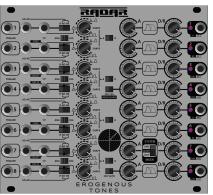
RADAR was designed to be a high density octal AD/AR envelope generator providing a variety of features and modes that you can work with. RADAR stands for (R)epeating, AD, or AR.
