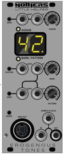
The ASSIGN setting is sent when a GATE is received or the SEND button to the left of the GATE is activated. When applying external CV, the ASSIGN knob becomes an attenuator to control the range of the signal coming in. There are 16 assign settings possible. Be sure to consult the Mother32 documentation for what those settings do. (6 is a lot of fun)
