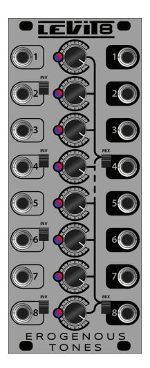
If you engage the CHANNEL4 MIX up, then OUTPUT 4 will be a MIX of 1,2,3 and 4. At the same time, the 1,2 and 3 OUTPUT will continue to pass through the associated INPUT. The same is true of 5,6,7 and 8.
